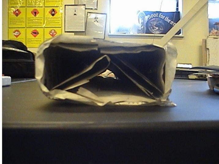
Wing X: By the time Wings 1 and 2 were finished, there was no time to create the large cylinder imperative for this wing and still meet the 3-wing minimum for testing. A compromise was made, and the shell was quickly stuffed with starch-coated balls of starched paper, a procedure that took less than 5 minutes, but resulted in a questionable wing.
